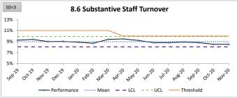
If the LCL is negative (less than zero) it is set to zero. If the UCL is greater than 100% it is set to 100%.
